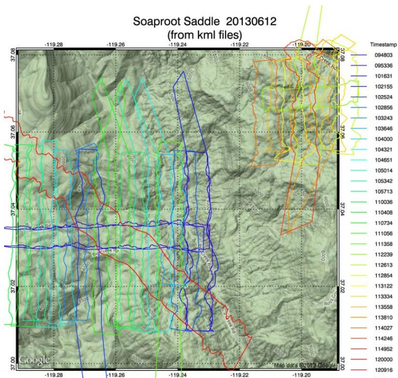
Figure 30: Flight tracks and spectrometer swaths for June 12 flight over Soaproot Saddle and KREW/Providence Creek
