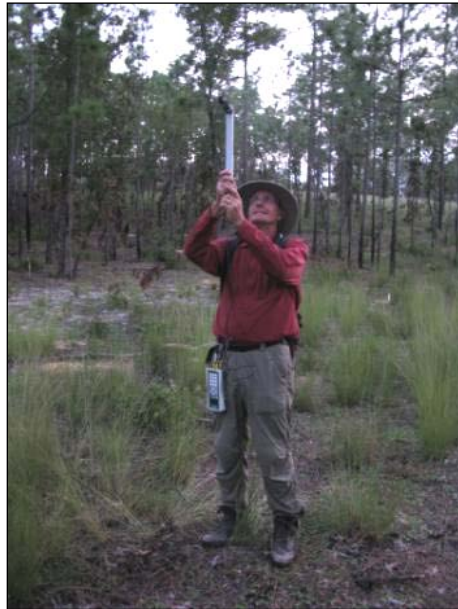
Figure 21. NEON Staff conducting LAI Measurements using the LICOR LAI-2200.
