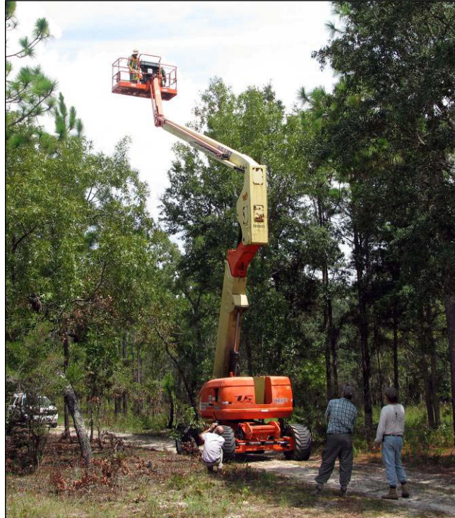
Figure 36. Above-canopy spectroscopic measurements at OSBS using the ASD FieldSpec instrument from atop an aerial boom.
