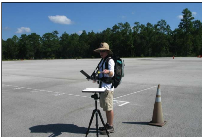
Figure 5. Reflectance reference measurement being made at the southern corner of the asphalt site.
