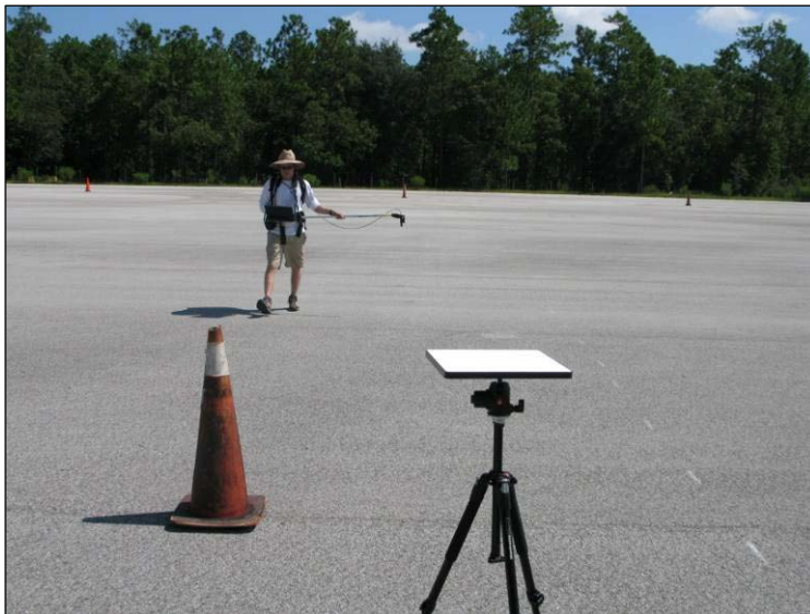
Figure 30. Surface reflectance measurements of the aged asphalt site
