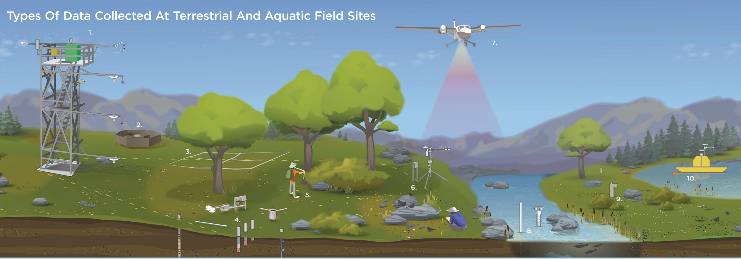
1. A flux tower collects atmospheric data at terrestrial sites.
