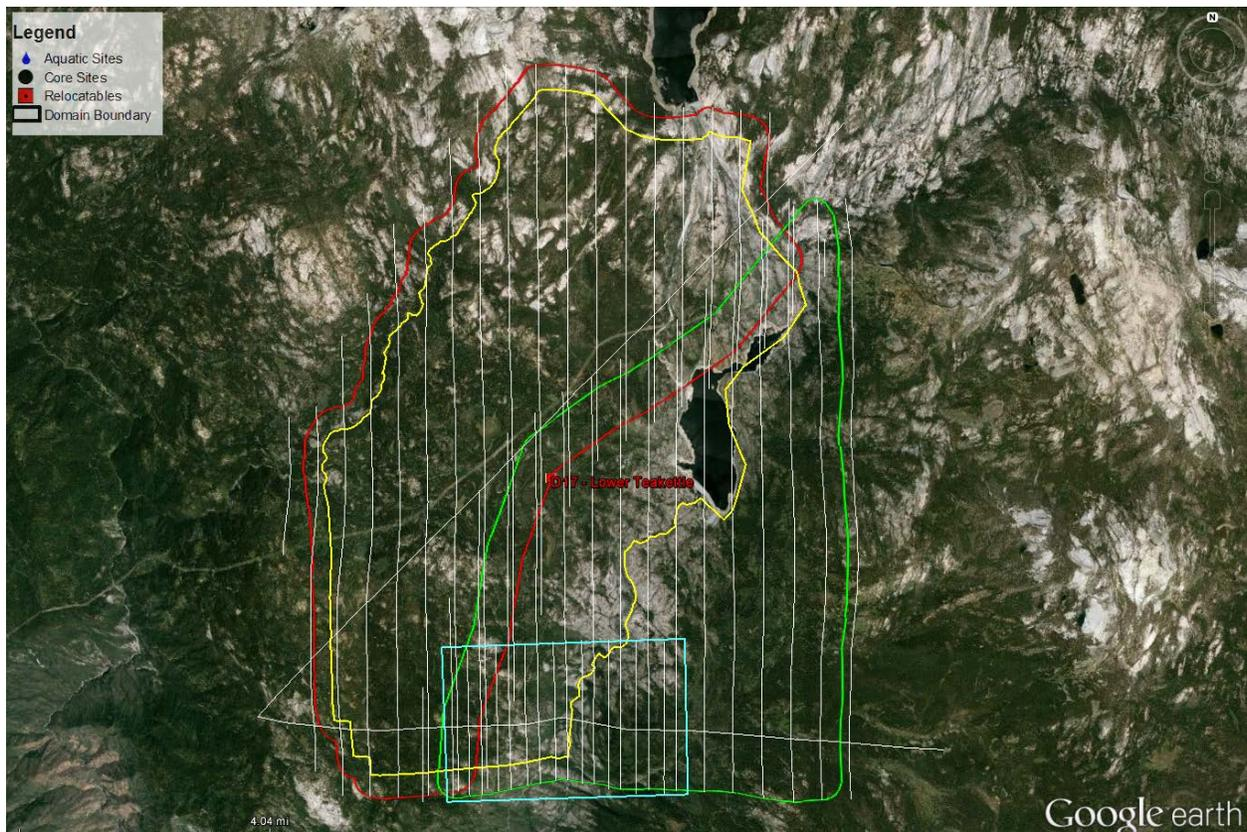
Figure 26: Flight lines for Teakettle (flight box 1=red; flight box 2=green; flight box 3=blue)
