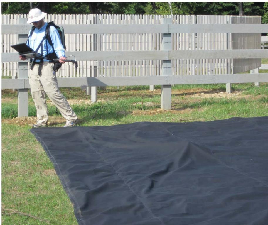
Figure 35: Measuring spectral reflectance with ASD field spectroradiometer over reference reflectance tarp.
