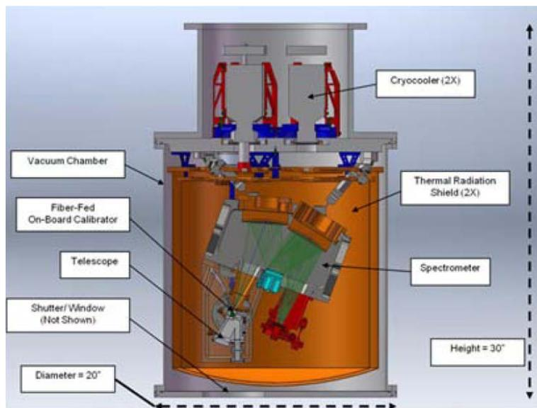
Figure 12: Schematic view of the NEON Imaging Spectrometer (NIS) showing major subsystems
