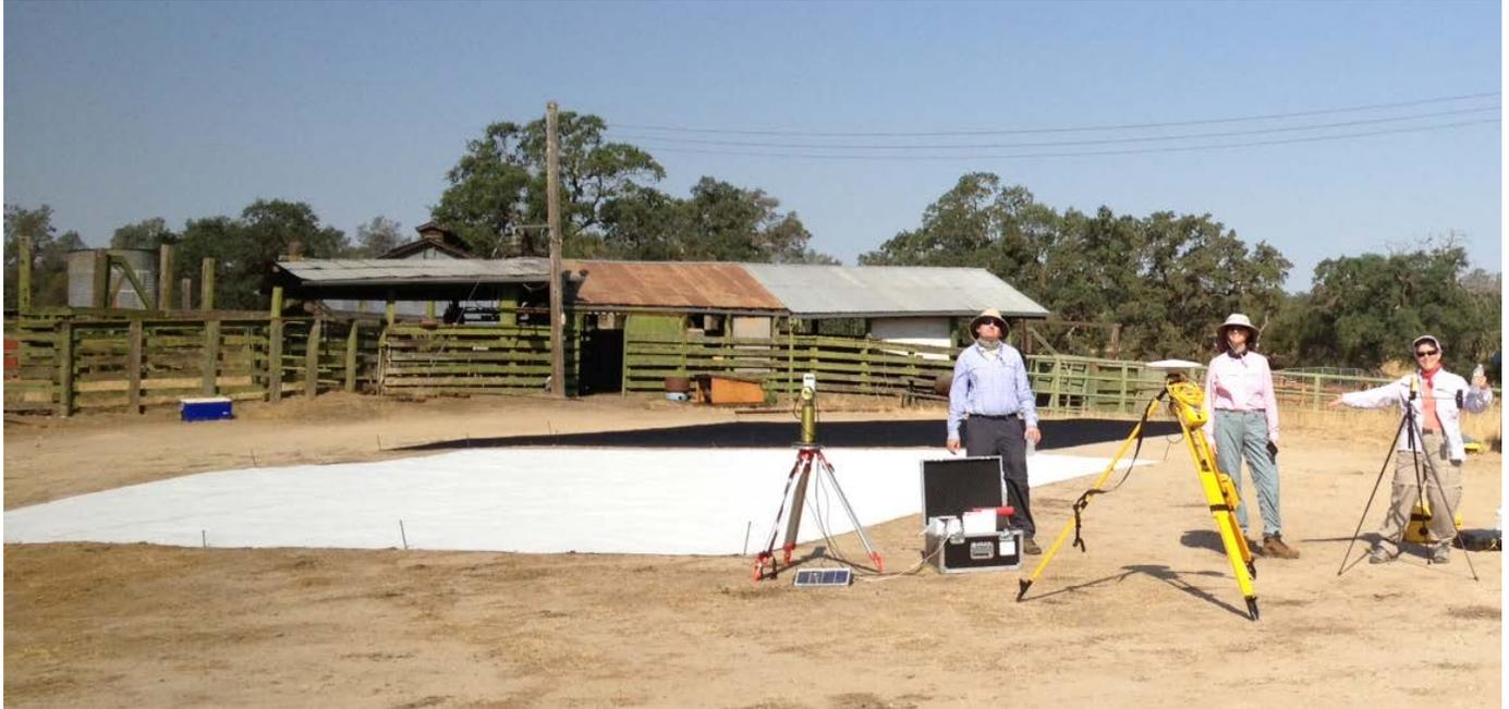
Figure 34: Setting up the CIMEL sun photometer (left), Trimble GPS base station (middle), Kestrel weather station (right) and Tracor tarp (behind) in SJER.
