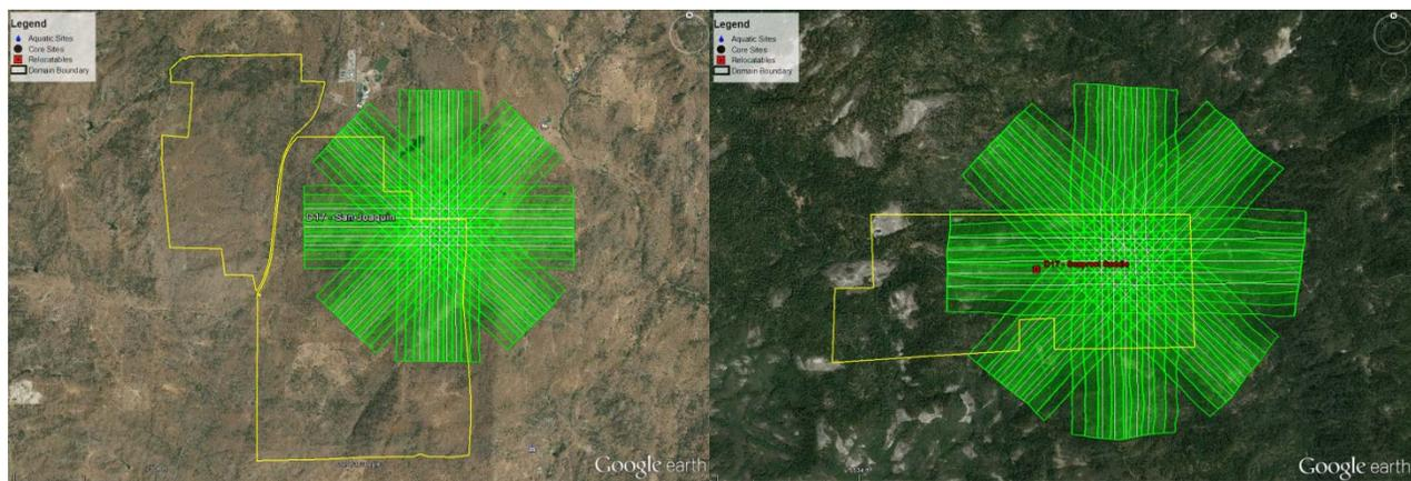
Figure 29: BRDF flight lines in SJER and Soaproot Saddle.
