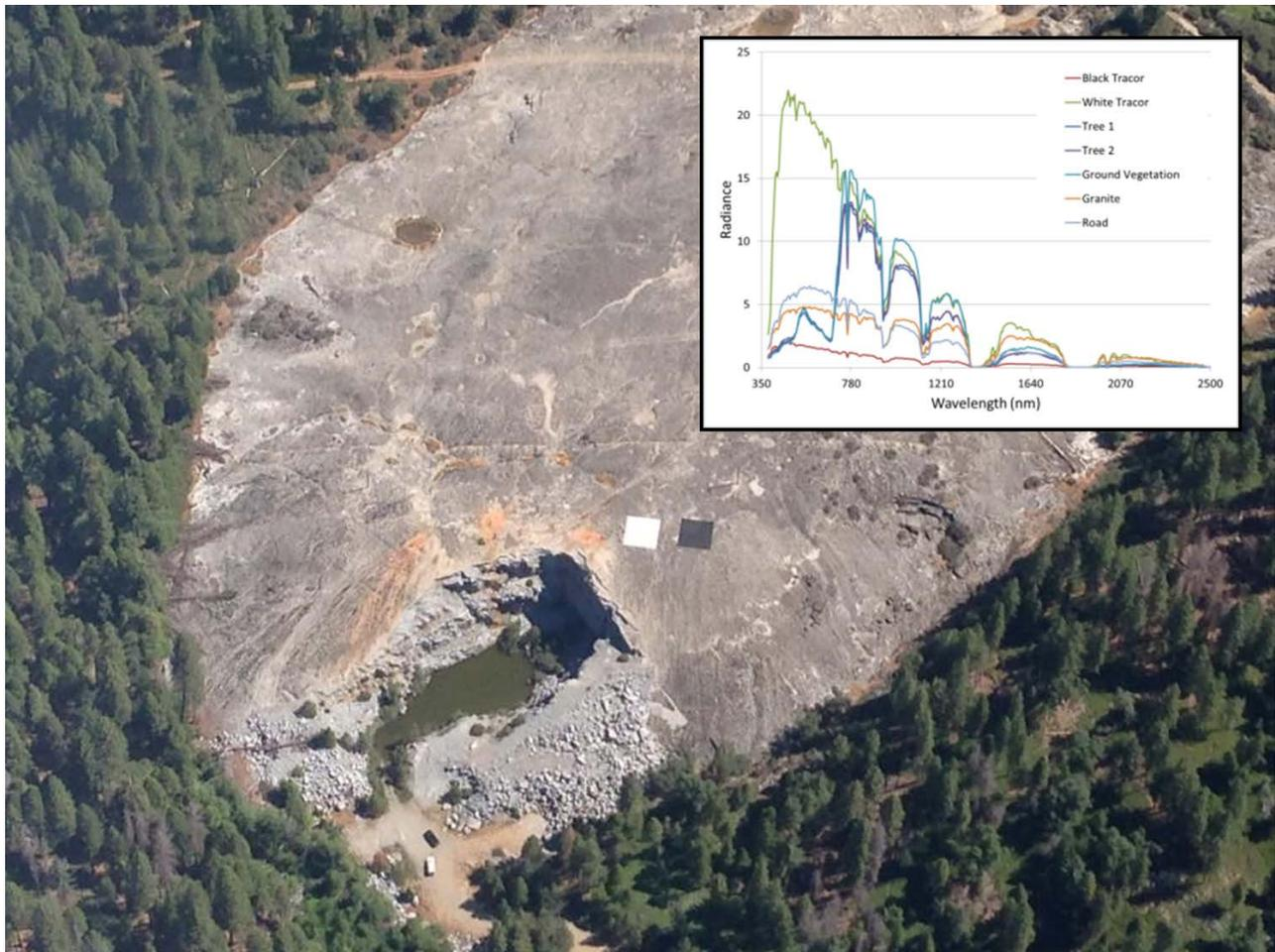
Figure 50: Tracor tarps used as reflectance calibration references. Note the two vehicles at the base of the rock outcropping at the lower left of the image.
