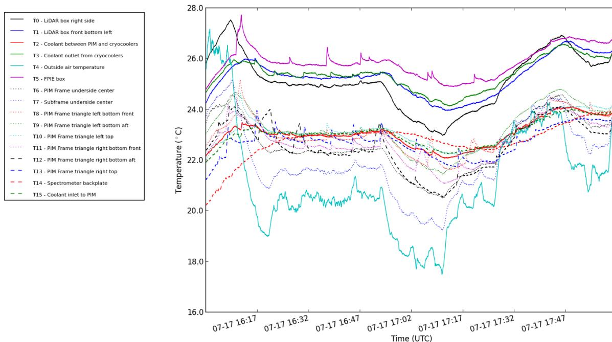
Figure 15: LiDAR and PIM remote monitoring software output
