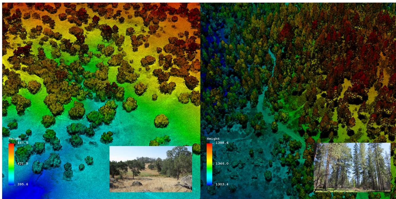
Figure 51: LiDAR point clouds of the San Joaquin Experimental Range (left) and Soaproot Saddle (right) NEON sites. The two sites have different horizontal and vertical 3D structures due to the differences in vegetation cover.
