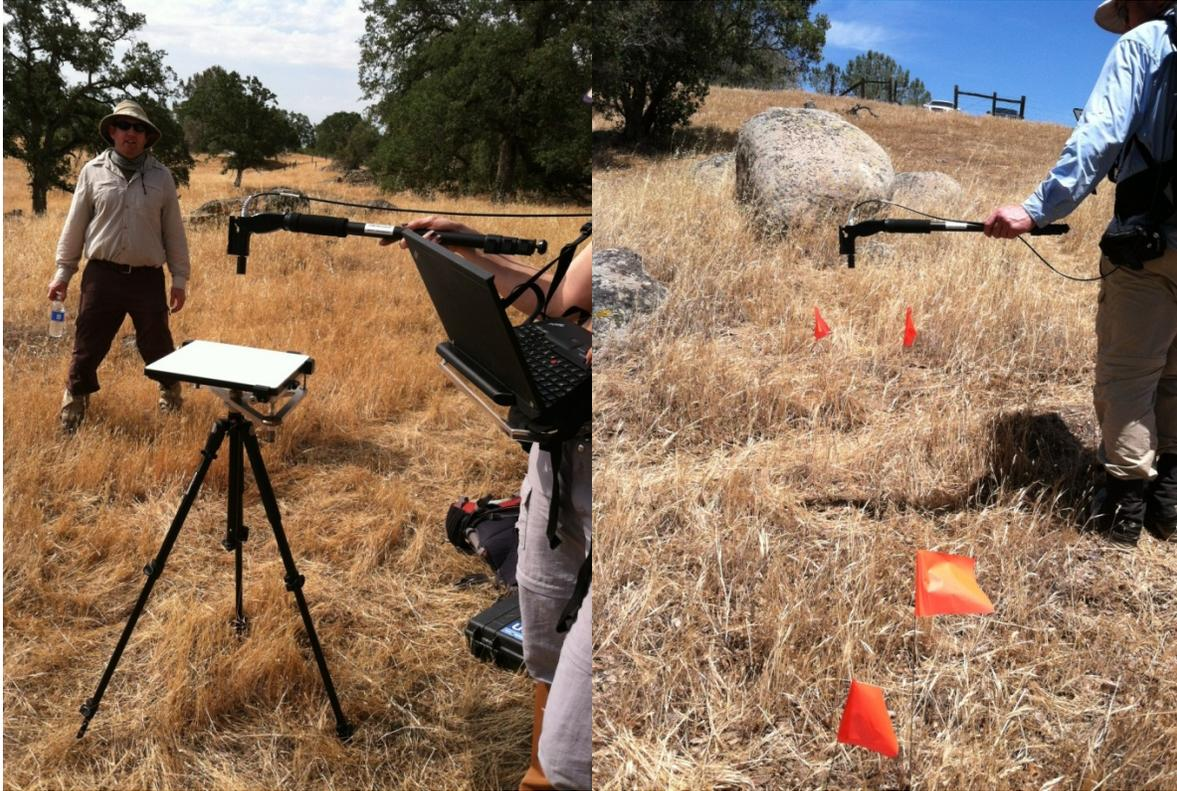
Figure 38: Transect Protocol: collecting reflectance data over the Spectralon panel (middle); collecting spectra over transect subplot (right)
