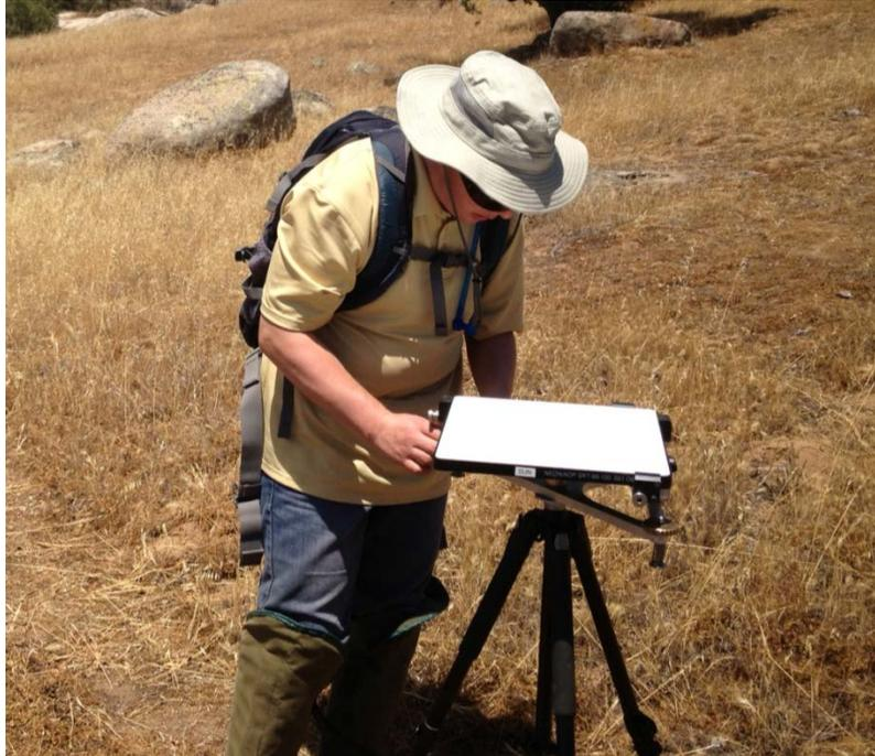
Figure 37: Preparing a Spectralon reflectance panel used to calibrate ASD measurements
