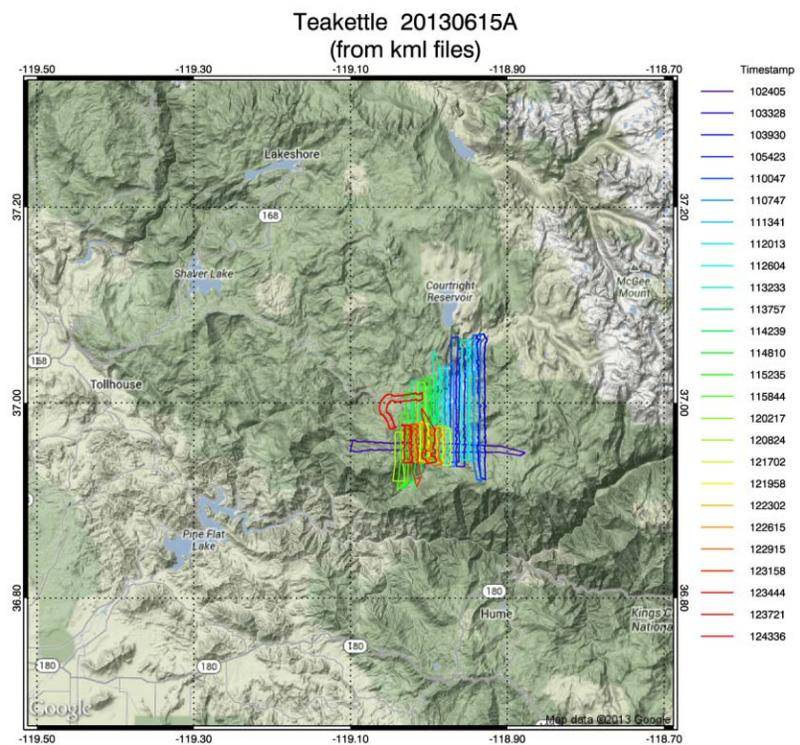
Figure 33: Flight tracks and spectrometer swaths for June 15 flight over Teakettle
