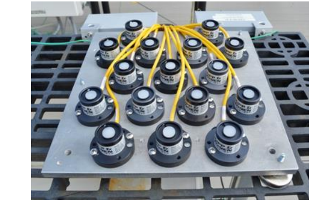
Figure 8. PSQ1 sensors compared to standardized sensor
