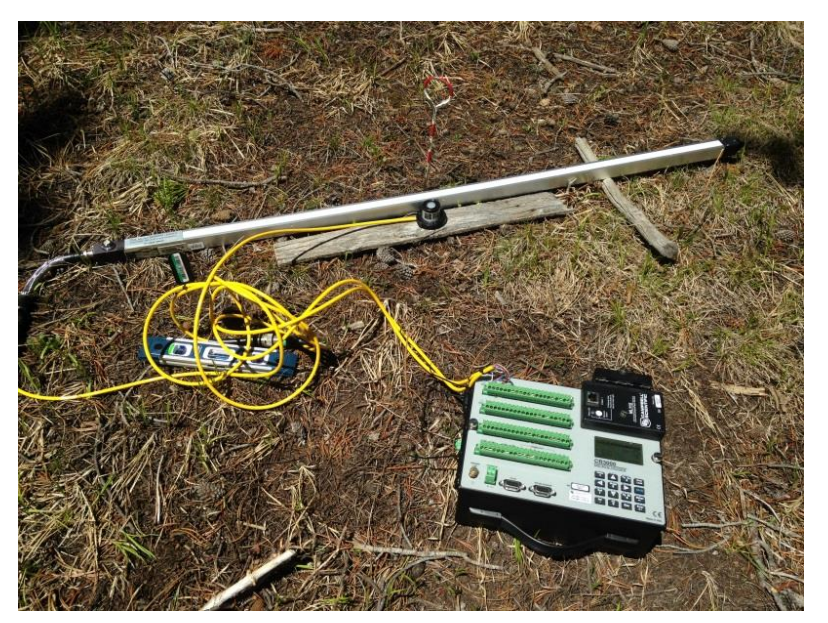
Figure 4. Transect system with a point sensor (PSQ1, Kipp & Zonen, Delft, Netherlands), line quantum sensor (LI-191SL, LI-COR Inc, Lincoln, NE) and a data logger (CR3000, Campbell Scientific, Logan, UT)
