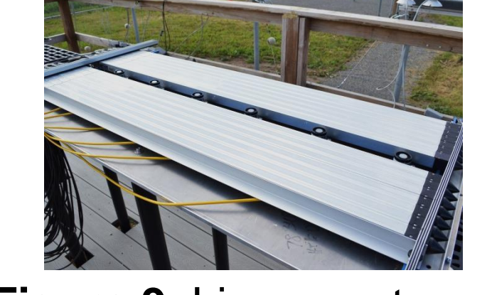
Figure 9. Line quantum sensors calibrated using six standardized point sensors
